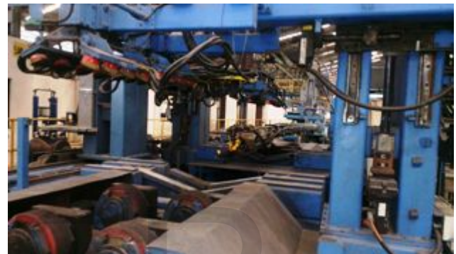
Figure 3 : SAW welding machine used for experimentation
